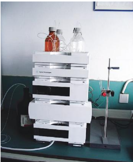
HPLC to analysis content of high molecular material, addition agent.
